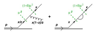
$$\frac{dq(x,\mu^2)}{d \ln \mu^2} = \frac{\alpha_s}{2\pi} \int_{x}^{1} dz \, p_{qq}(z) \, \frac{q(x/z,\mu^2)}{z} - \frac{\alpha_s}{2\pi} \int_{0}^{1} dz \, p_{qq}(z) \, q(x,\mu^2)$$
