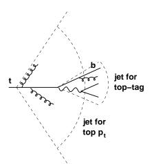
Within inner cone  $\sim \frac{2m_t}{p_t}$  (dead cone) you have the top-quark decay products, but no radiation from top ideal for reconstructing top mass
